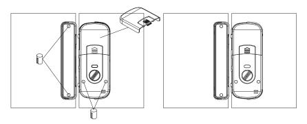
4. Left-open/right-open direction adjustment method
